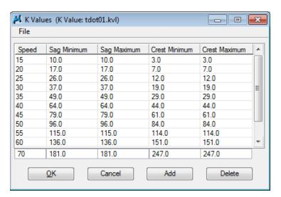
If you need to reset this table, in the K Values dialog select the drop down option  $File \rightarrow Open$ , navigate to the folder C:\Users\Public\Geopak Standards and load the desired file. Click on the OK button once settings are made.
