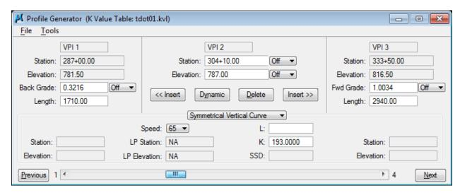
9) Make sure the curve type at the bottom is **set** to **Symmetrical** and **set** the **Design Speed** to **60**. The K value is automatically read from our table and a curve length of 92.72 is computed.
