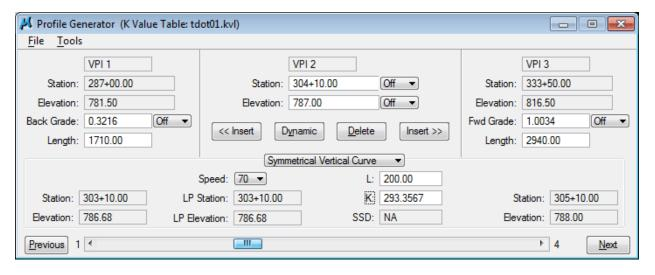
The new curve length is used to calculate a new K value which is used with our K value table to indicate that we are now meeting 70 mph vertical design speed criteria.
